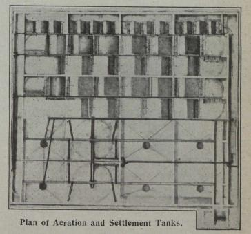
gallons (120,000 cubic feet) of sewage per day could be settled in the first set of settling tanks if the suspended solids in effluent were to be kept down below 4 parts per 100,000, it was decided to alter the slopes of the second set of tanks and utilize them in the same way. This has now been done, affording an extra capacity of 40,000 gallons (6,400 cubic feet) for settling purposes.
