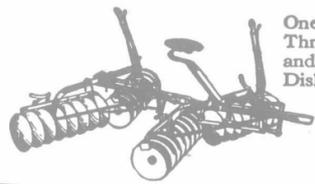
will thoroughly cultivate and pulverize any soil. One Harrow is Out Throw; the other is In Throw. They are simply constructed, rigid and durable. The Gangs are flexible and the Disk Plates are so designed that they "hang" right into the soil. Bissell Harrows are built in sizes and weights suitable for horse or tractor use. Write Dept. W for free catalogue. 98
