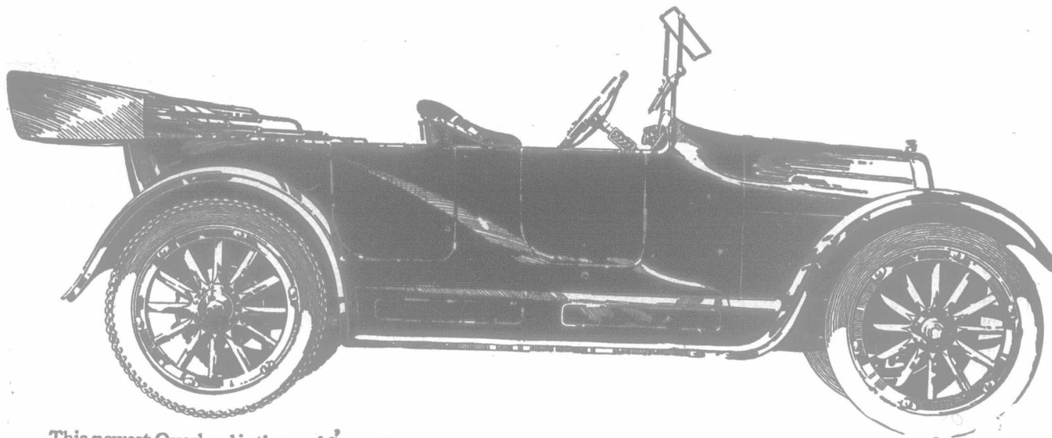
This newest Overland is the world's most powerful low-priced car. It has a 31½ horsepower en bloc motor that is a perfect marvel for speed, power and endurance. By increasing the bore of the motor from 3¼" to 3¾" we are able to offer a power plant which at 1950 R. P. M. develops full 31½ horsepower.
