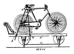
tially as and for the purpose set forth. 3rd. The construction, arrangement and combination of parts constituting my improved apparatus for teaching or practicing the riding of a velocipede, substantially as set forth and as illustrated in the accompanying drawings.
