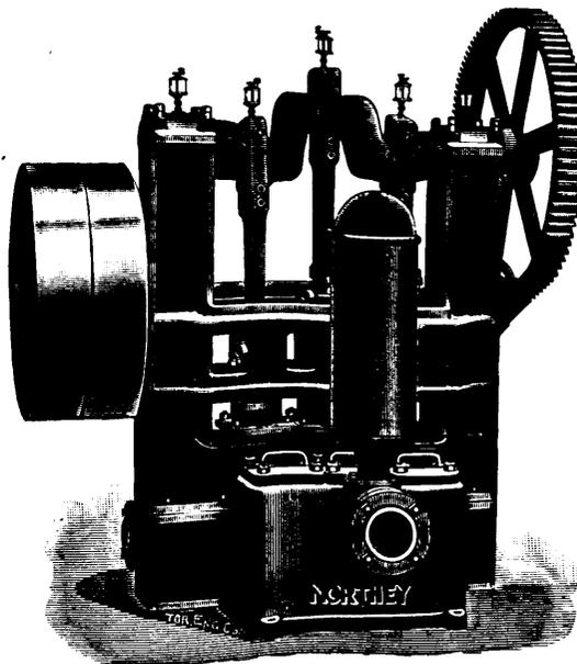
We illustrate in this advertisement a typical Pump for Mine Work. This is our Triplex Power Pump, fitted with tight and loose pulleys as shown in cut. It is the regular Triplex type with the three cranks 120 degrees apart; crankshaft and connecting rods are of steel; gears machine-cut from the solid; plungers of brass and all details carefully worked out. This Pump is especially adapted for service with Electricity as the motor power.
