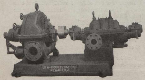
Ask for bulletin describing this Terry Steam-Turbine driven boiler-feed centrifugal or the same type of pump with motor drive—also other types of centrifugal pumping machinery.
