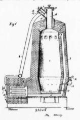
5. A vertical coking chamber, a fire box and flues leading from said box up around said coking chamber and side changing into said chamber below the level of the top of a normal charge, substantially as described.
