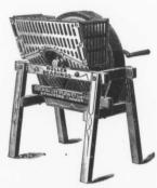
Cockshutt Cylinder Pulper with reversible knives and easy running roller bearings. Grinds up the roots entirely. No large pieces left. New device keeps the roots right on the knives while working. Extra large drive wheel—strong at every point—a tried and proven favorite.
