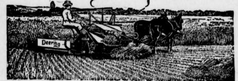
THESE Deering binder features appeal to the farmer. The elevator, open at the rear, delivers the grain properly to the binding attachment. Because the elevator projects ahead of the knife it delivers grain to the binder deck straight. A third packer reaches up close to the top of the elevator and delivers the grain to the other two packers. A third discharge arm keeps the bound sheaves free from unbound grain.
