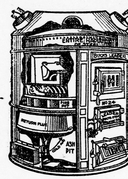
Sectional View of Buck's Leader Furnace
