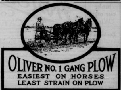
WHEN plowing with an Oliver No. 1 gang plow, the load is equalized at a point which brings the draft strain equally on both beams and equally on each horse. There are no unnecessary side strains on the beams and therefore no tendency for joint bolts to work loose. There is no tendency to pull the plow out of adjustment, therefore it runs easier, strains bearings less, lasts longer and is easier on horses. This feature is found only on Oliver plows.
