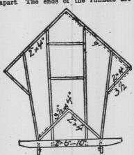
PLAN OF SELF FEEDER. rounded at both ends, so that the feeder may be pulled either way. Nine 2 by 4 joists each 9 feet long are bolted on to the runners about two feet apart. These joists are then fastened together by 2 by 6 joists which project over the runners far enough to support the feed trough.
