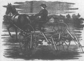
Experience has demonstrated the fact that a good HAY TEDDER that will thoroughly spread long, heavy grass, taking it up from the bottom, tossing it gently into the air, and leaving it upon the ground in a light, fleecy condition, enables the farmer to take advantage of fair weather and at least twice the quantity of hay can be segured, in better condition, than when allowed to remain in the swath.
