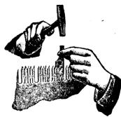
Place the Set on the point of tooth as shown in the above cut, and strike a very light blow.
