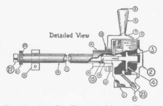
The minimum burner flame Pilot and the Independent Pilot must be properly adjusted by the person installing the Range.
