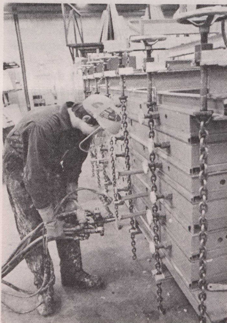
Daniel Leclerc of Foster Refrigerator injects urethane foam between panels. This foam is the insulating agent for all Foster refrigeration units.
