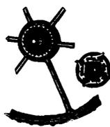
**BRANTFORD MOWER DRIVE WHEELS** are broad face and high enough to ensure light running. Four Pawls work in 27 teeth.
