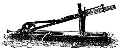
PRIZE at the Provincial Exhibition held in Toronto in 1862. It raises the Saw and zigs up the log by 18 own action, and is so simple that a child can operate it. They are not hable to get out of order, and are warranted capable of cutting from 70 to 80 cords of Wood per day.
