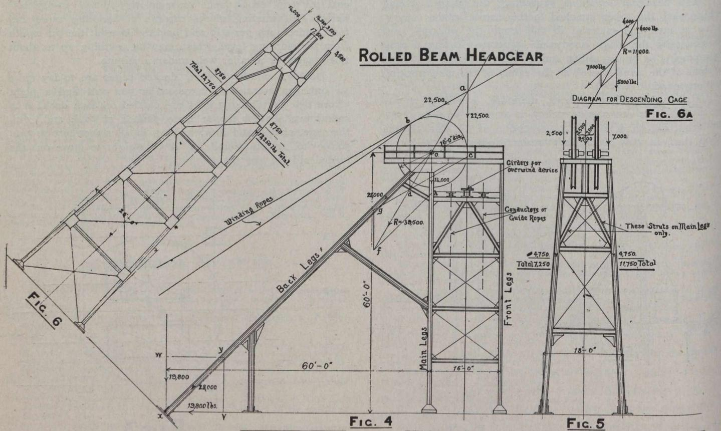
winding ropes, are all made of steel, and the diameter will be anything from one inch to an inch and a half.
