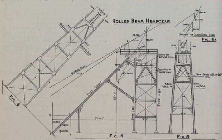
winding ropes, are all made of steel, and the diameter will be anything from one inch to an inch and a half.
