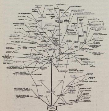
Fig. 1.—Products of Coal Tar, with Special Reference to American Conditions.
