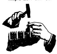
Directions. - Place the Set on the point of tooth as shown in the above cut, and strike a very light blow with a tack hammer. If you require more set, file the tooth with more bevel. If you follow directions you can not make a mistake. Be sure and not strike too hard a blow, and it will set the bardest saw
