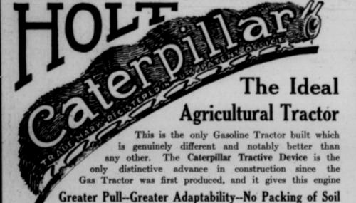
THE CATERPILLAR LAYS ITS OWN STEEL TRACK AND RUNS ON IT LIKE A LOCOMOTIVE. This track gives from 2,000 to 4,000 square inches of bearing surface, depending on the width of track. The weight of engine is evenly distributed over this whole surface, giving it the lightest bearing per square inch and the most powerful tractive grip of any engine built.
