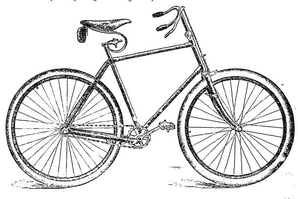
Our work is made from the best Steel Forgings and cold drawn Steel Tubing, not an ounce of cast metal being used.
