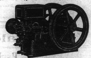
The Jumbo is an exceptionally good engine for hoisting, sawing, etc. Positive starting magneto eliminates batteries and coils and their attend-
