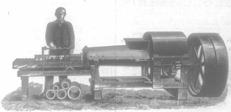
No. 2 machine makes tile from two and a-half to eight inches. No. 1 machine makes tile from two and a-half to twelve inches. Both sold on approbation. Satisfaction guaranteed. A full line of Brick and Tile Machinery and Supplies, Kiln Bands, Kiln Doors, Grates, everything necessary for a first-class outfit. For full particulars address
