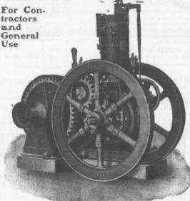
Equipped with Variable Speed Device. Gan be started or stopped in a moment.
