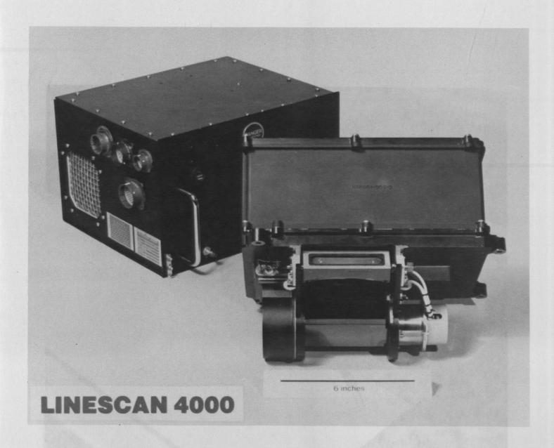
Figure 12. Linescan 4000 infrared linescan system. The system is compact and can be used on a wide range of platforms. It provides horizon-to-horizon coverage, electronic roll stabilization, real time video output and can be down-linked to a ground station. It has a multi-element mercury cadmium telluride detector operating in the 8 to  $14 \mu m$  waveband and a closed cycle helium detector cooling system. (Courtesy of Vinten Military Systems Ltd.)
