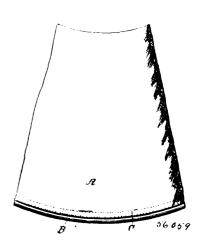
a skirt having its lower edge doubled back, of a skirt binding consisting of an upwardly doubled strip of chamois skin sewed to the doubled edge of the skirt, and a supplemental binding having a doubled edge secured to the chamois skin.
