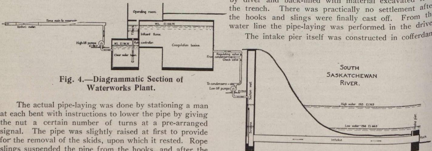
Fig. 4.—Diagrammatic Section of Waterworks Plant.
