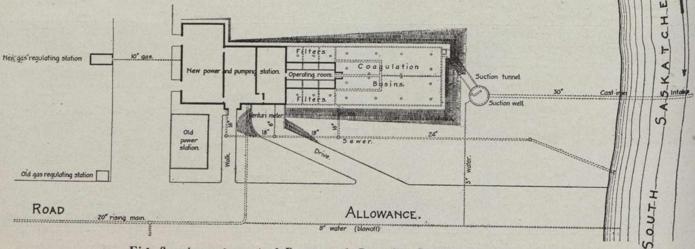
Fig. 3.—Arrangement of Power and Pumping Station and Filter Plant.
