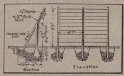
remove. About five years ago a start was made toward the construction of snow fences along the most unprotected sections of the line, following the design shown in the accompanying illustration. Since then the whole line has been so protected, with great success.
