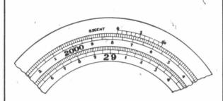
The division lines on vernier are numbered from 0 to 10 if altitude scale be in 10 feet divisions, and 0 to 20 if scaled for 20 feet.
