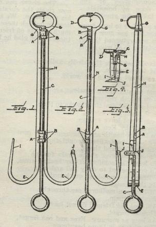
to the ends of bars H. These bars are provided with hinge knuckles, A. B, by means of which they are hinged together. The hinge pin is preferably formed by the handle, C. of the knife, D. This knife is of semiannular form, as shown, and when rotated moves in shear fashion past the inner faces of the rings, G. G. The outer ends of the
