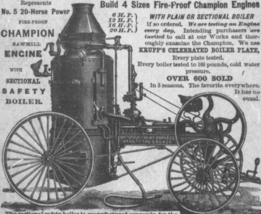
The sectional safety boiler is manufactured expressly for the "North West" trade. This boiler is so arranged that it is readily taken apart in sections enabling purchasers to clean thoroughly every part of it and prevent burning out. We know from experience this is absolutely necessary with the alkaline waters of the great Western prairies. Largely used by the Pacific Railway Company and all the large Colonization and Rancho Companies.
