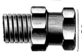
Screwed for Standard Iron Pipe Thread.
