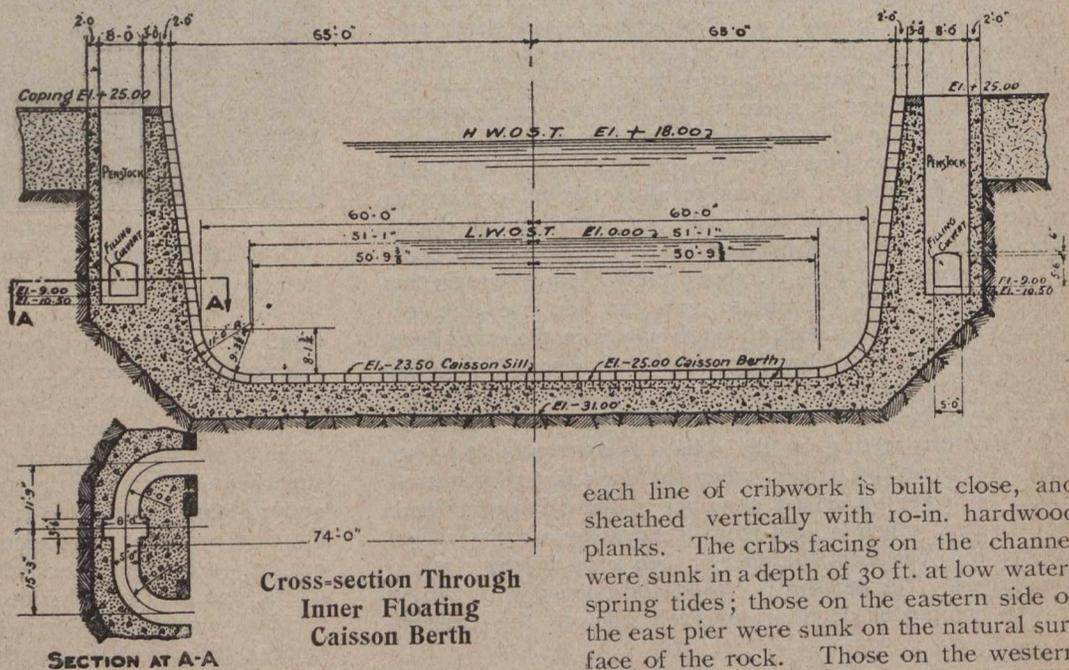
Cross-section Through Inner Floating Caisson Berth
