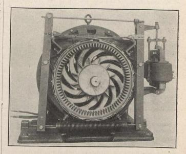
cycles. The braking action depends on the contraction of a coiled steel spring.
