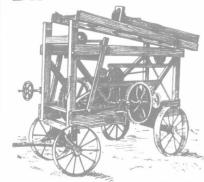
HE Noiseless Well Drilling Machine is the term usually applied to The Standard when compared to other makes, with their incessant rattle and clang. They are compactly constructed and their mechanism is built of iron and steel-not wood
