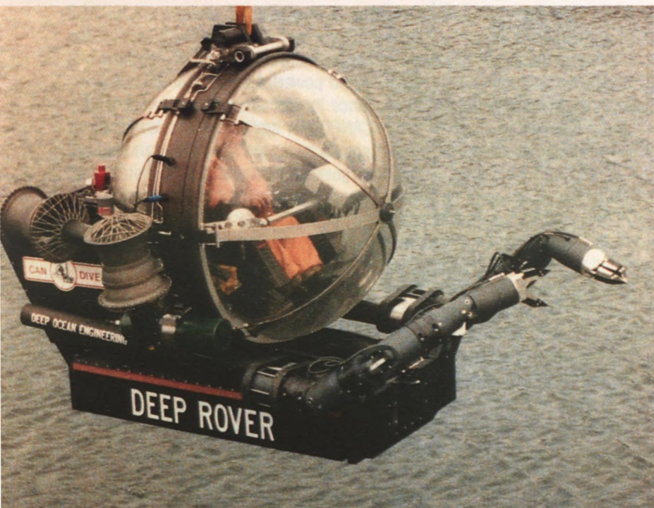
Can-Dive's Deep Rover submersible is a state-of-the-art system for depths to 915 metres.
