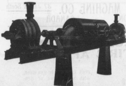
Two Worthington 3-Stage Turbine and McCormack Water Wheels, built for Port Arthur, Ont., Water Works, 1440 gal. per minute against 350 ft. head.
