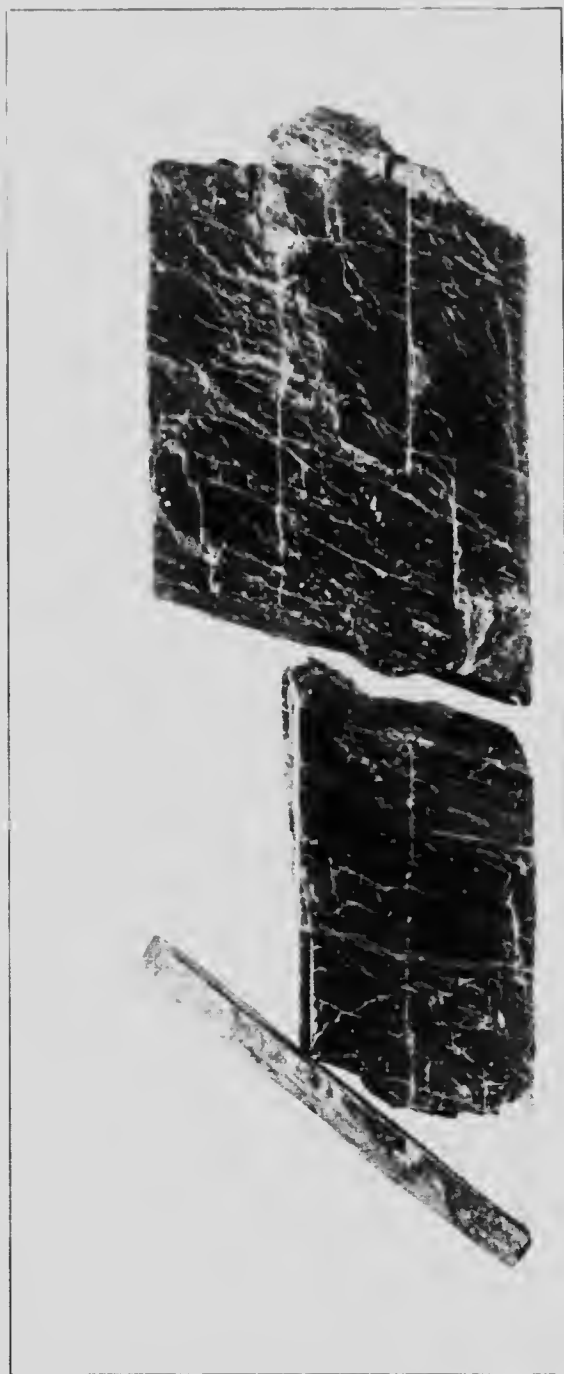
Cleavage pieces of microcline feldspar of characteristic reddish-brown colour, from quarry of the Kingstons Feldspar and Mining Company, Bedford township, Ont
