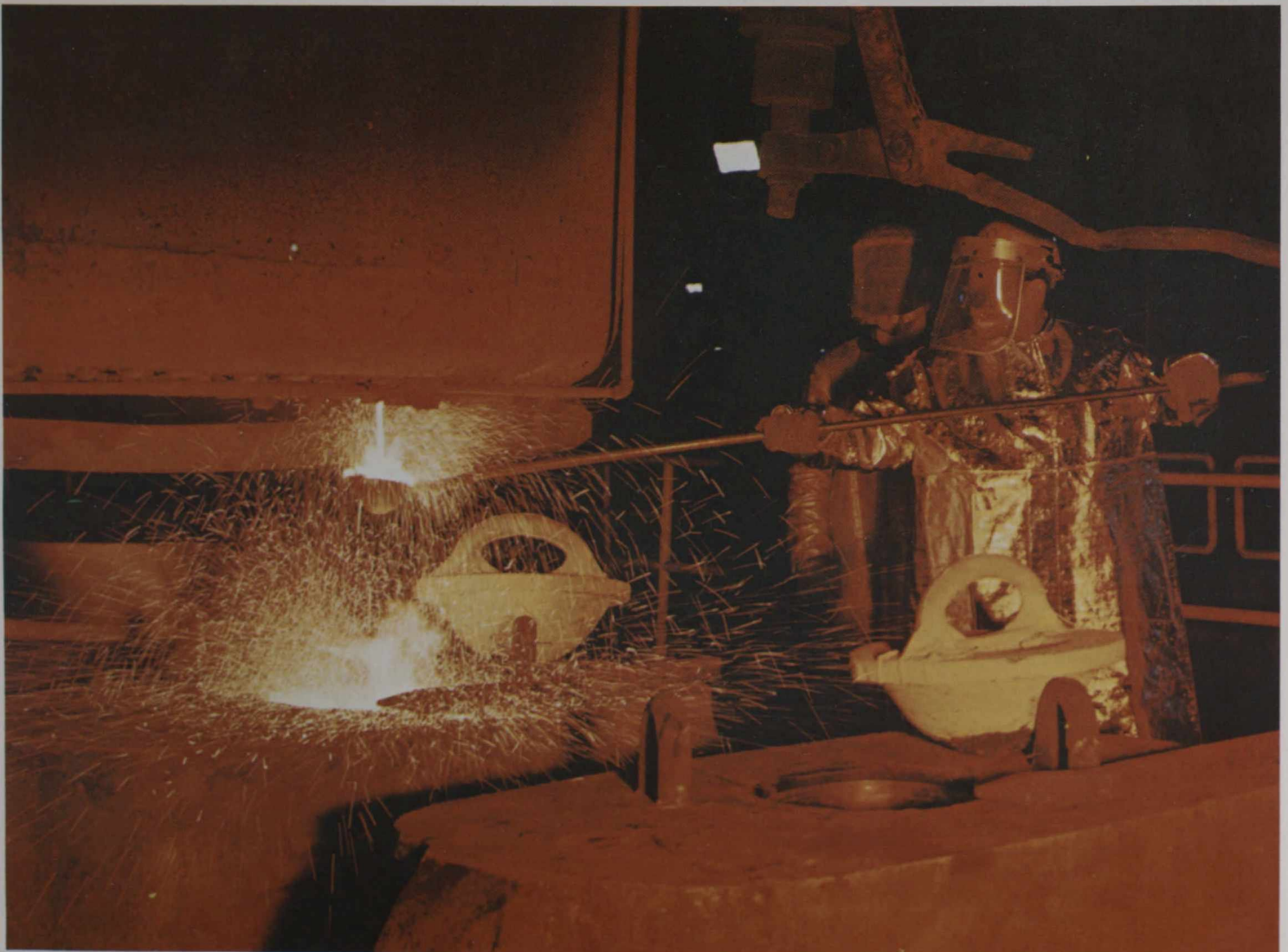
Below: Teeming on the oxygen melt shop floor. The average weight of ingots poured during this operation is 10 tons.
