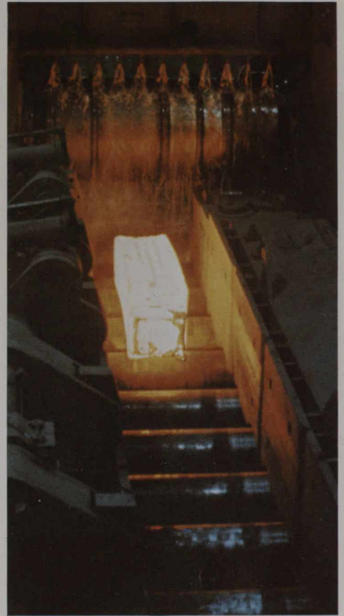
Below: Teeming on the oxygen melt shop floor. The average weight of ingots poured during this operation is 10 tons.
