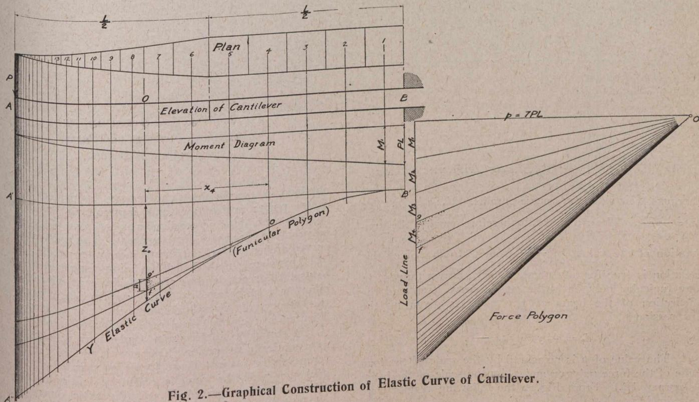
Fig. 2.—Graphical Construction of Elastic Curve of Cantilever.
