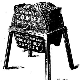
Being the only Double Root Cutter manufactured, and is noted for being a Safe, Rapid, and Easy Machine, and one which sells at sight after a careful inspection, as it will either pulp coarse or fine, or slice hysection, as it will entry purpose or me, or size by simply turning over the centre grate and turning crank the reverse way. It is considered in either capacity superior to any single machines, and has taken first prize at every fair where exhibited, where prizes were given.
