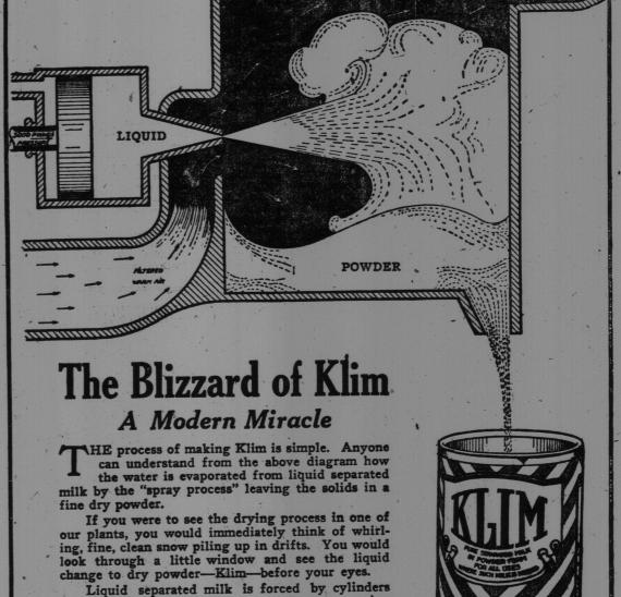
Liquid separated milk is forced by cylinders through tiny pinholes by great pressure, coming out in the form of a cloud or mist, just as from a huge atomizer. This fine spray enters a large square room through which are blowing strong currents of filtered warm air. The spray of liquid is whirled they the spray just as you have seen the wind blow about the room just as you have seen the wind blow
