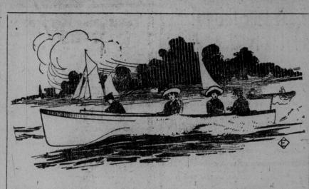
It is fitted with the EATON 5 h.p. reversible engine installed in forward end of cockpit with solid propeller and shaft and has a speed of eight miles and hour; seating 10 people. Depth at bow is 40 in.; draught, 18 in.; beam 4 ft. 9 in. Stem, stern, deadwood and engine bed all white oak. Complete launch fitted with cushions delivered to your nearest railway station in Ontario without. charge. Price .... 275.00
