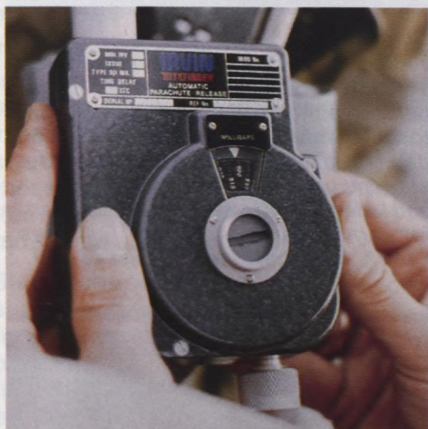
FF-2 Hite Finder automatic parachute release mechanism for military freefall parachuting.
