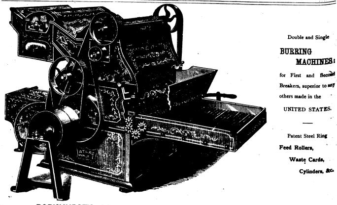
PARKHURST'S PATENT DOUBLE CYLINDER BURRING PICKER, For Pisking, Burring, and Dusting all grades of Wool. Recent Improvements, including a bester attached to the spout for the purpose of more theroad mixing and eleaning the Wool without injury to the staple, make it superior to any other machine now in use. Manufactured only by
