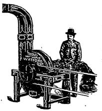
OUR PATENT BLOWER ATTACHMENT as a Silo filler is all OUR FAILENT BLOWER ATTACHMENT as a Sho mier is an right. It has been thoroughly tested at 20, 25 and 30 feet, and will elevate green corn 40 feet if necessary. We are so satisfied that our Blower Elevator is the coming machine that we offer to forfeit the machine if we fail to elevate the desired height. In the language of one customer "the Blower has come to stay."
