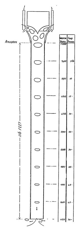
McLeod of McGill University. The first three tests were made on the 7th August and the last three were made on the 13th of August, 1896. Column (2) gives the quantity of water in cubic feet per minute flowing through the compressor; column (3) the available head
